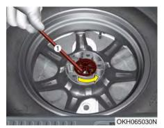
If it is hard to loosen the tire holddown wing bolt by a hand, you can loosen it easily using the Jack handle. 1.Put the Jack handle (1) into the inside of tire hold-down wing bolt.
