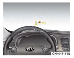
The head up display is a transparent display which projects a shadow of some information of the instrument cluster and navigation on the windshield glass.
