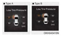
When the tire pressure monitoring system warning indicators are illuminated and warning message displayed on the cluster LCD display, one or more of your tires is significantly under-inflated. The low tire pressure position telltale light will indicate which tire is significantly under-inflated by illuminating the corresponding position light.
