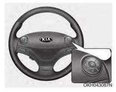
The LCD display modes can be changed by using the control buttons on the steering wheel.
