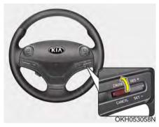
Move the lever up (to CRUISE). (the CRUISE indicator light in the instrument cluster will go off).
