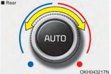
The temperature will increase to the maximum (HI) by pushing the up ( $\land$ ) button (for front) or turn the knob to the right (for rear).
