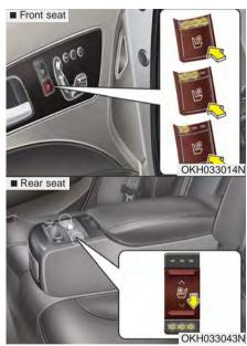
The air ventilation is provided to cool the seats during hot weather by blowing air through small vent holes on the surface of the seats and seatbacks. While the engine is running, press the switch to cool the seat.
