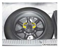
Turn the tire hold-down wing bolt counterclockwise.
