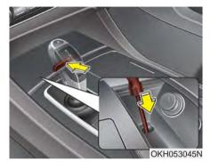
You can shift into [N] by using the driver if the jump starting is impossible to do.
