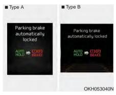
If the EPB is applied while Auto Hold is activated because of ESC (Electronic Stability Control) signal, a warning will sound and a message will appear.
