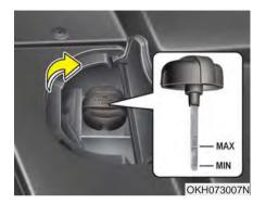
With the vehicle on level ground, check the fluid level in the power steering reservoir periodically. The fluid should be between MAX and MIN marks on the side of the gauge at the normal temperature.
