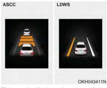
This mode displays the state of the Advanced Smart Cruise Control (ASCC) or Lane Departure Warning System (LDWS).
