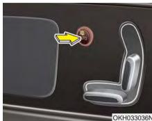
Your vehicle features an easy access system to provide convenient access for rear passengers. When opening the rear door, the rear seats will move rearward automatically to provide easier access for passengers. This easy access system will operate only when the control switch is in "ON" position.
