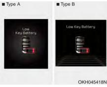
This warning message illuminates if the battery of the smart key is discharged when the Engine Start/Stop Button changes to the OFF position.
