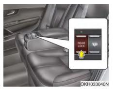
You can activate or deactivate the rear seat control, rear audio control and climate control by using the REAR LOCK button on the rear armrest or "System Settings" in the AVN (Audio, Video, and Navigation).
