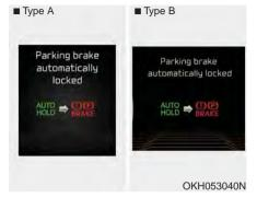
When the EPB is applied from Auto Hold, the notice will illuminate on the LCD display. Also, warning chime sounds once.
