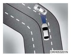
Your vehicle speed can be reduced due to a vehicle in the adjacent lane. Adjust your vehicle speed by depressing the brake pedal according to the road condition ahead and driving condition. Apply the accelerator pedal and select the appropriate set speed. Check to be sure that the road conditions permit safe operation of the ASCC.
