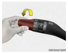
When the light switch is in the headlight position, the head, tail and license lights will turn ON.
