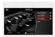
If your vehicle is equipped with the auto defogging system, it is automatically activated when the conditions are met
