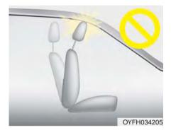
If you recline the seatback towards the front with the headrest and seat cushion raised, the headrest may come in contact with the sunvisor or other parts of the vehicle.
