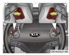
The paddle shifter is available when the shift lever is in the D (Drive) position or the sports mode.
