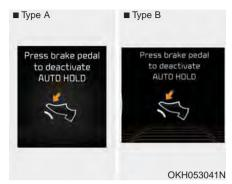
If it is impossible to apply EPB from Auto Hold, the notice will illuminate on the LCD display. Also, warning chime sounds once. In that time, apply the brake pedal.
