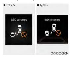
The message will appear to notify the driver if there are foreign substances on the rear bumper or it is hot near the rear bumper. The light on the switch and the system will turn off automatically.
