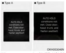
When you press the [AUTO HOLD] switch, if the driver door, engine hood and trunk are not closed or the driver seat belt is not fastened, the notice will illuminate on the LCD display. Also warning chime sounds once. In that time, press the [AUTO HOLD] button after closing the driver door, engine hood and trunk and fastening the seat belt.
