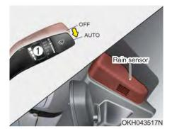
The rain sensor located on the upper end of the windshield glass senses the amount of rainfall and controls the wiping cycle for the proper interval.
