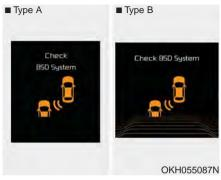
If the system does not work properly, a warning message will appear and the light on the switch will turn off. The system will turn off automatically.
