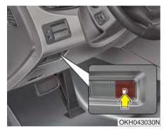
The fuel filler lid must be opened from inside the vehicle by pushing the fuel filler lid opener.
