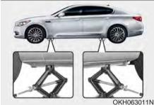
8. Place the jack at the front (1) or rear (2) jacking position closest to the tire you are changing. Place the jack at the designated locations under the frame. The jacking positions are plates welded to the frame with two tabs and a raised dot to index with the jack.
