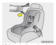
3.Pull the shoulder portion of the seat belt all the way out. When the shoulder portion of the seat belt is fully extended, it will shift the retractor to the "Auto Lock" (child restraint) mode.
