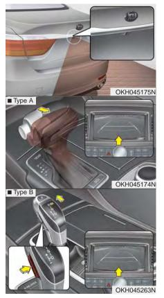
The Parking Guide System is not a substitute for proper and safe parking procedures. The Parking Guide System may not detect every object surrounding the vehicle. Always drive safely and use caution when parking. The Parking Guide System (PGS) will activate when the back-up light is ON with the Engine Start/Stop Button ON and the shift lever in the R (Reverse) position.
