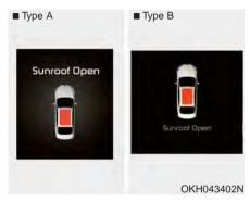
If the driver turns off the engine when the sunroof is not fully closed, the warning chime will sound for a few seconds and a warning message will appear on the LCD display.
