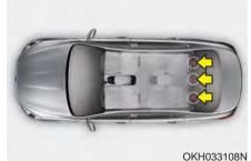
Child restraint hook holders are located on the package tray.
