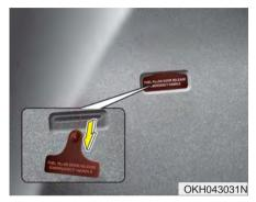
If the fuel filler lid does not open using the remote fuel filler lid release, you can open it manually by pulling the handle outward slightly.
