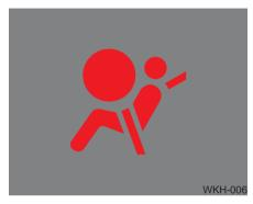
The purpose of the air bag warning light in your instrument panel is to alert you of a potential problem with your air bag - Supplemental Restraint System (SRS).
