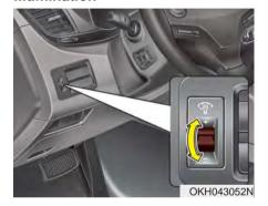
The brightness of the instrument panel illumination can be adjusted by pressing the illumination control buttons ("+" or "-") when the Engine Start/Stop Button is ON or the tale lights are turned on.
