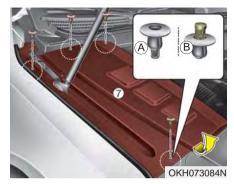
(A): for assemble, (B): for remove
