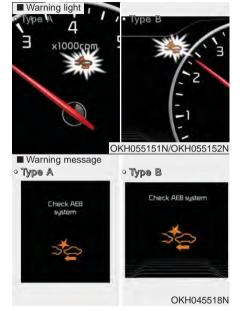
When the AEB system is turned off, the AEB warning light turns on. (Warning message does not come on.)
