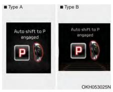
7. While stopping in [D], [R] and [M], when you get off the vehicle, the warning will be illuminated for your safety and the shifting is automatically changed to [P].
