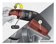
When the light switch is in the AUTO light position, the taillights and headlights will be turned ON or OFF automatically depending on the amount of light outside the vehicle.
