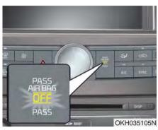
Your vehicle is equipped with an occupant detection system in the front passenger's seat.
