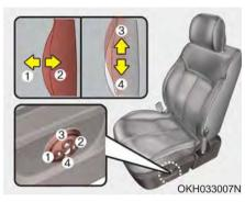
The lumbar support can be adjusted by pressing the lumbar support switch on the side of the front seat. Press the front portion of the switch (1) to increase support, or the rear portion of the switch (2), to decrease support. Move the support position up and down by pressing the switch (3) or (4). Release the switch once the seat reaches the desired position.
