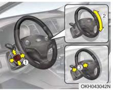
Adjust the steering wheel angle (2) and position (3) with the knob (1) on the steering column. Move the steering wheel, so it points toward your chest, not toward your face. Make sure you can see the instrument panel warning lights and gauges. After adjusting, push the steering wheel both up and down to be certain it is locked in position. Always adjust the position of the steering wheel before driving.
