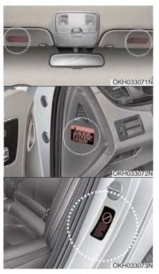
Air bag warning labels, some required by the U.S. National Highway Traffic Safety Administration (NHTSA), are attached to alert the driver and passengers of potential risks of the air bag system.
