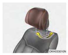
The headrest may be adjusted forward or rearward by pulling the lower part of the headrest forward or rearward to the desired detent in the direction of the arrow. Adjust the headrest so that it properly supports the head and neck.
