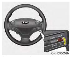
3.Lever must be moved down (to SET-) prior to setting any desired speed. The Set speed in the instrument cluster will illuminate. Release the accelerator at the same time. The desired speed will automatically be maintained.
