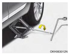
9.Insert the jack handle into the jack and turn it clockwise, raising the vehicle until the tire just clears the ground. This measurement is approximately 1.2 in (30 mm).
