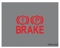
Check the brake warning light by placing the Engine Start/Stop button to the ON position. (do not start the engine). This light will be illuminated when the parking brake is applied with the Engine Start/Stop button in the START or ON position.
