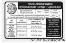
The label located on the driver's door sill gives the original tire size, cold tire pressures recommended for your vehicle, the number of people that can be in your vehicle and vehicle capacity weight.
