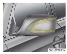
If the light bulb does not operate, have the vehicle checked by an authorized K900 Kia dealer. A skilled technician should check or repair the side repeater light, for it may damage related electrical parts and housing of outside mirror.
