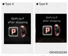
5. When you shift into [P], if the vehicle speed is high, warning will be illuminated. Stop the vehicle at safe area and shift into [P].
