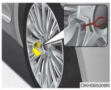
6.Insert the tool (1) into the hole and pull out the wheel cap.
