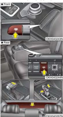
To raise the rear curtain, depress the button. To lower the rear curtain, depress the button again.
