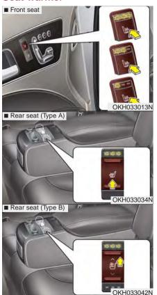
The seat warmer is provided to warm the seats during cold weather. With the engine start/stop button in the ON position, push the switch to warm the seat.
