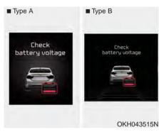
This warning message illuminates if the battery voltage is abnormally low, or the battery has poor performance. In this case, have your vehicle inspected by an authorized K900 Kia dealer.
