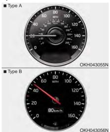
The speedometer indicates the speed of the vehicle and is calibrated in miles per hour (mph) and/or kilometers per hour (km/h).
