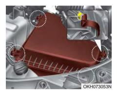
7.Loosen the air cleaner cover attaching clips and open the cover.8.Wipe the inside of the air cleaner.
