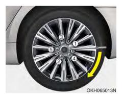
Then position the wrench as shown in the drawing and tighten the wheel nuts. Be sure the socket is seated completely over the nut. Do not stand on the wrench handle or use an extension pipe over the wrench handle. Go around the wheel tightening every other nut until they are all tight. Then double-check each nut for tightness. After changing wheels, have an authorized K900 Kia dealer tighten the wheel nuts to their proper torque as soon as possible.
