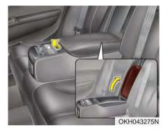
To open the rear seat storage, pull up the lever.
