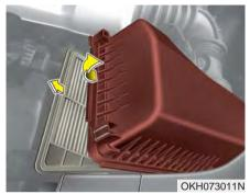
9.Replace the air cleaner filter.10. Lock the cover with the cover attaching clips.
