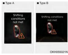
3.If the shifting condition is not matched by high engine RPM or high vehicle speed, the warning will be illuminated. When you reduce the engine RPM or vehicle speed, the shifting will be operated.
