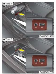
If your vehicle has an aux and/or USB(universal serial bus) port or iPod® port, you can use an aux port to connect audio devices and a USB port to plug in a USB, and an iPod® port to plug in an iPod®.
