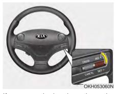
If any method other than the CRUISE lever was used to cancel cruising speed and the system is still activated, the most recent set speed will automatically resume when you move the lever up (to RES+).
