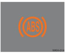
The ABS warning light will stay on for approximately 3 seconds after the Engine Start/Stop button is ON. During that time, the ABS will go through self-diagnosis and the light will go off if everything is normal. If the light stays on, you may have a problem with your ABS but your regular brakes will work normally. Contact an authorized K900 Kia dealer as soon as possible.
