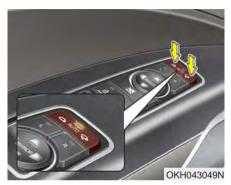
The outside rearview mirror can be folded or unfolded by pressing the switch as below.
