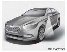
When all the doors (and trunk) are locked and closed, the puddle lamp will come on for about 15 seconds if any of the below is performed.
