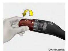
When the light switch is in the parking light position, the tail and license lights will turn ON.
