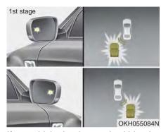
If a vehicle is detected within the boundary of the system, a warning light will illuminate on the outside rearview mirror and the head up display.
