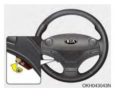
When the Engine Start/Stop Button is in the ON position, press the heated steering wheel button to warm the steering wheel. The indicator on the button will illuminate.
