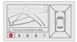
**Camera View Modes** – To change camera view modes, press the icons shown below on the navigation screen to select the mode.
