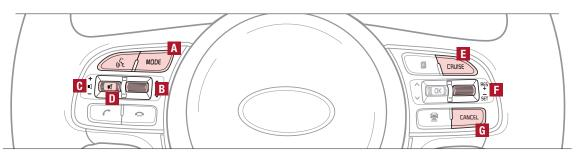
A Audio MODE button: Press to cycle through FM 1-2/AM/SAT 1-3/CD/ USB/Aux/iPod®
