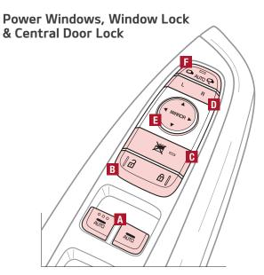
A Pull/Press to operate Driver's and Front Passenger's Windows Auto-Up/Down\*
