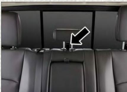
**Tether Strap Loop With Head Restraint
