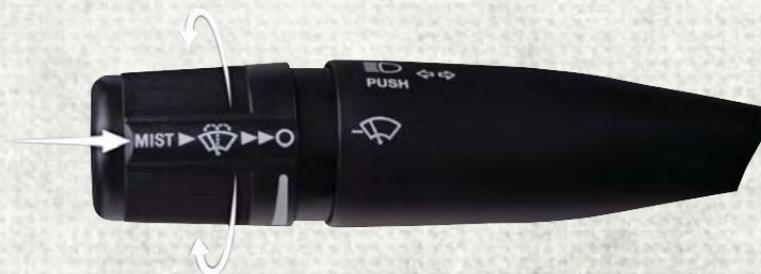
Turn Signal/Wiper/Washer/High Beam Lever
