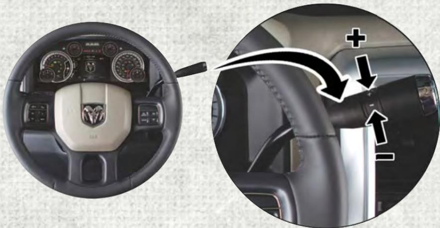
ERS Control On The Gear Selector
