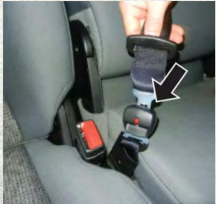
**Inserting Latch Plate**
