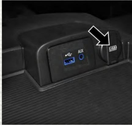
**Power Outlet (USB Charge Only Port) — Storage Compartment**
