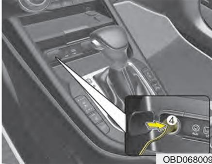
8. Connect the compressor to the vehicle power outlet using the cable and connectors (4).
