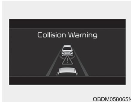
This warning message appears on the LCD display with a warning chime.
