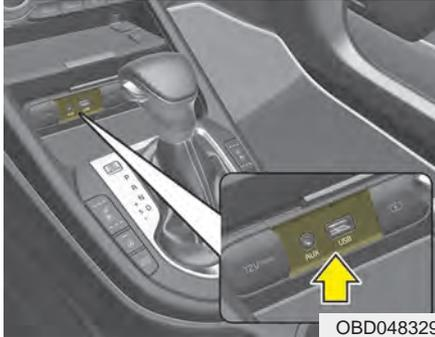
You can use the AUX port to connect audio devices and the USB port to plug in a USB device or iPod®.
