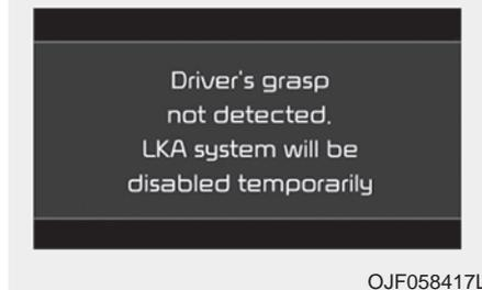
If the driver takes hands off the steering wheel for several seconds while the LKA is activated, the system will warn the driver.
