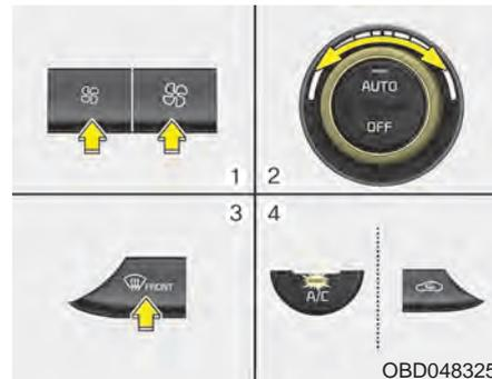
1. Set the fan speed to the desired position.
