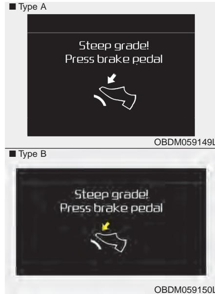
This warning message is displayed when the vehicle is driven slowly on a grade and the vehicle detects that the brake pedal is not applied.
