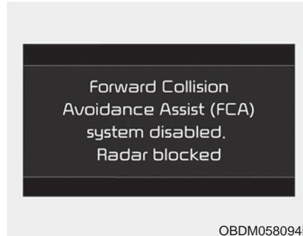
When the sensor is covered or the sensor lens is dirty with foreign substances, such as snow or rain, the FCA system may not be able to detect vehicles. In this situation, a warning message ("Forward Collision-Avoidance Assist (FCA) system disabled. Radar blocked") will appear to notify the driver. Remove the foreign substances to allow the FCA system to function properly.
