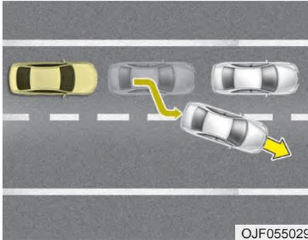
When driving in stop-and-go traffic, and a stopped vehicle in front of you merges out of the lane, the FCA system may not immediately detect the new vehicle that is now in front of you. In this situation, you must maintain a safe braking distance, and if necessary, depress the brake pedal to reduce your driving speed in order to maintain a safe distance.
