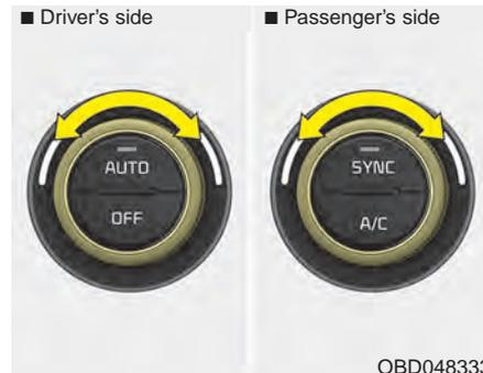
The temperature will increase to the maximum (HI) by turning the knob all the way to the right.
