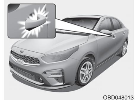
When all the doors (and tailgate) are locked and closed, the door handle lamp will come on for about 15 seconds if any of the below is performed.
