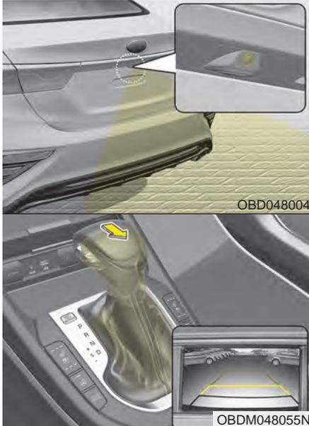
The rear view monitor will activate with the ignition switch ON and the shift lever in the R (Reverse) position. The system is a supplemental system that shows the area behind the vehicle through the audio screen while backing up.
