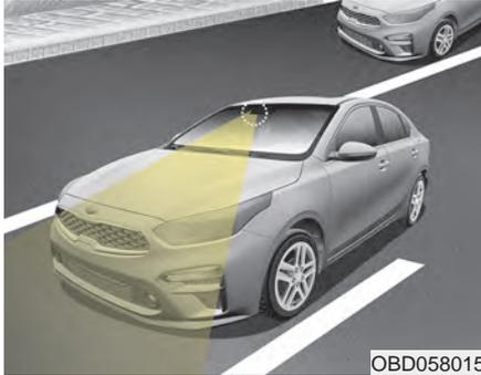
The Lane Keeping Assist system is designed to detect the lane markers on the road with a front view camera at the front windshield, and assists the driver's steering to help keep the vehicle in the lanes.
