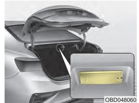
The trunk room lamp comes on when the trunk is opened.
