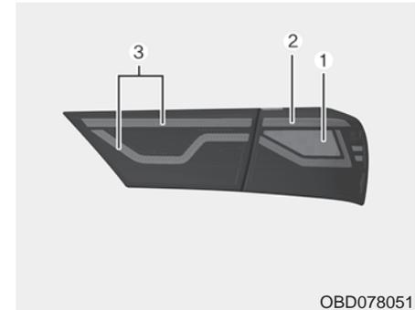
If the stop and tail lamp (LED) (1,2,3) does not operate, have the vehicle checked by an authorized Kia dealer. The LED lamp cannot be replaced as a single component because it is an integrated unit. The LED lamp has to be replaced with the unit.
