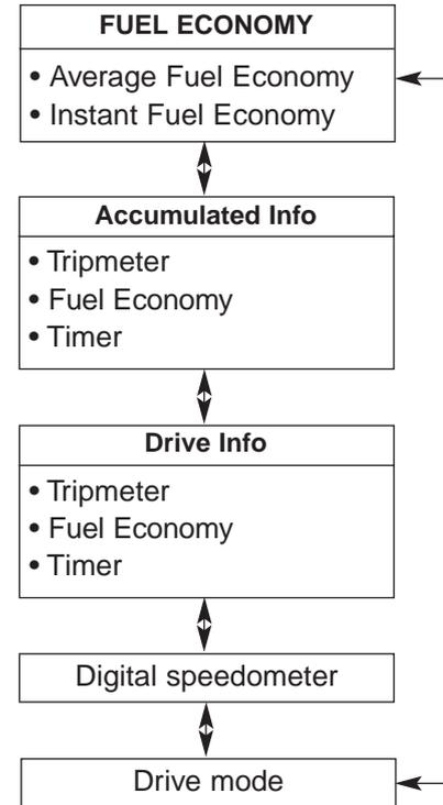
To change the trip mode, scroll the MOVE scroll switch (^/∨) or press the TRIP button in the trip computer mode.
