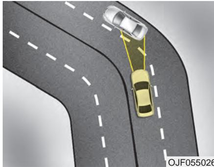
The FCA system may recognize a vehicle in an adjacent lane when driving on a curved road. In this situation, the system may apply the brake. Always pay attention to road and driving conditions while driving. If necessary, depress the brake pedal to reduce your driving speed in order to maintain a safe distance. Also, when necessary, you may depress the accelerator pedal to prevent the system from unnecessarily decelerating your vehicle. Always check the traffic conditions around the vehicle.
