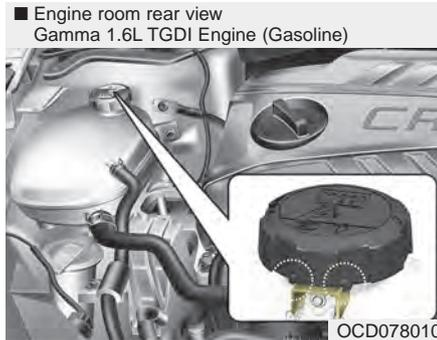
1. Make sure that the tiny protrusions inside the coolant cap are securely interlocked.
