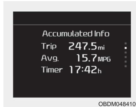
Displays accumulated information starting from a mileage/fuel efficiency/time default point.
