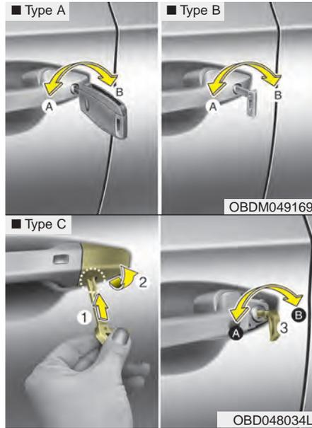
To remove the cover (if equipped, for type C) :
