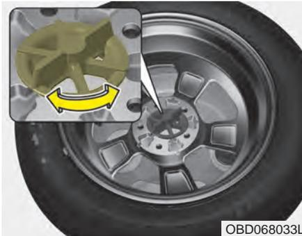
Turn the tire hold-down wing bolt counterclockwise to remove.
