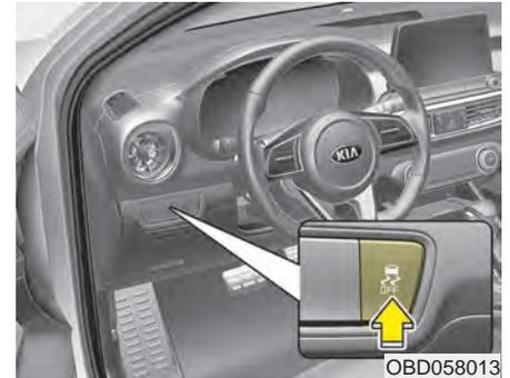
The Electronic Stability control (ESC) system is designed to stabilize the vehicle during cornering maneuvers. ESC checks where you are steering and where the vehicle is actually going. ESC applies the brakes on individual wheels and intervenes with the engine management system to stabilize the vehicle.
