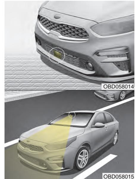
By detecting the vehicle or pedestrian ahead of the vehicle, the sensor helps to operate the Forward Collision-Avoidance Assist when the vehicle is at risk of a collision.
