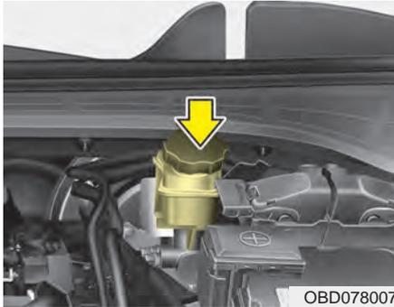
Check the fluid level in the reservoir periodically. The fluid level should be between the MAX (Maximum) and MIN (Minimum) marks on the side of the reservoir.
