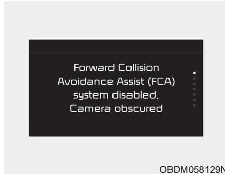
When the sensor is covered or the sensor lens is dirty with foreign substances, such as snow or rain, the FCA system may not be able to detect vehicles. In this situation, a warning message ("Forward Collision-Avoidance Assist (FCA) system disabled. Camera blocked") will appear to notify the driver. Remove the foreign substances to allow the FCA system to function properly.
