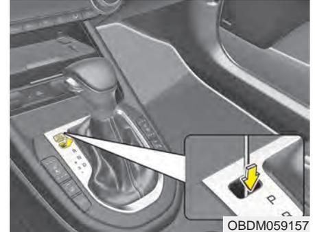
If the shift lever cannot be moved from the P (Park) position into R (Reverse) position with the brake pedal depressed, continue depressing the brake, then do the following:
