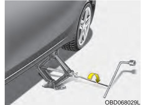
8. Insert the wheel lug nut wrench into the jack and turn it clockwise, raising the vehicle until the tire just clears the ground. This measurement is approximately 1 in. (30 mm).
