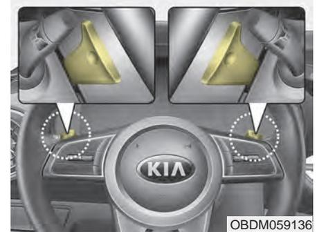
The paddle shifter is available when the shift lever is in the D (Drive) position or the manual mode.
