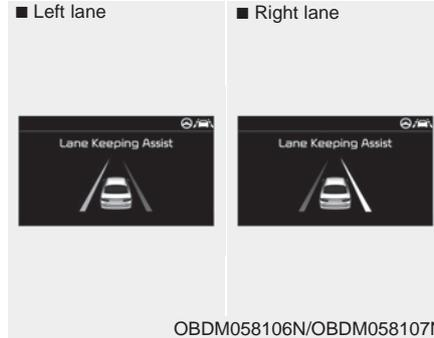
If the vehicle leaves a lane, the lane marker you cross will blink on the LCD display.
