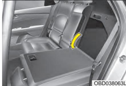
3. Pull out the seatback locking knob(1) in the trunk, then fold the seat toward the front of the vehicle.
