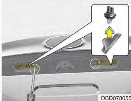
1. Remove the lamp assembly by using a flat-blade screwdriver.
