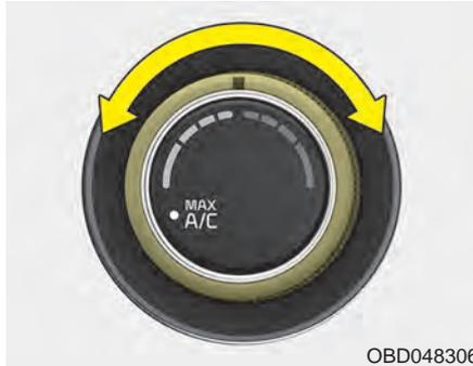
The temperature control knob allows you to control the temperature of the air flowing from the ventilation system. To change the air temperature in the passenger compartment, turn the knob to the right for warm and hot air, or to the left for cooler air.
