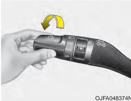
When the light switch is in the parking light position, the tail and license lights will turn ON.
