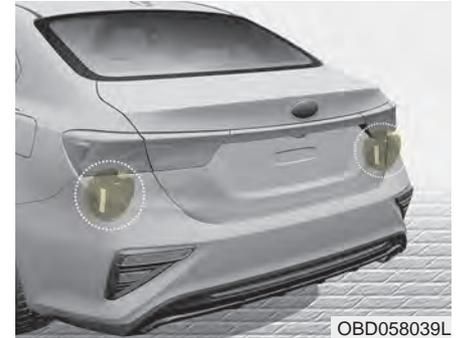
The sensors are located inside the rear bumper.
