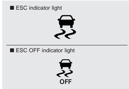
When the ignition switch is turned to ON, the indicator light illuminates, then goes off if the ESC system is operating normally.
