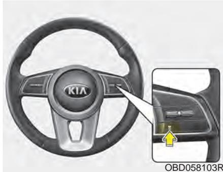
This function allows you to program the vehicle to maintain a relative distance to the vehicle ahead without depressing the accelerator pedal or brake pedal.
