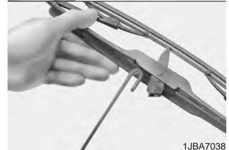
2. Compress the clip and slide the blade assembly downward.
