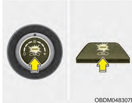
The air intake control is used to select the outside (fresh) air position or recirculated air position. To change the air intake control position, press the control button.
