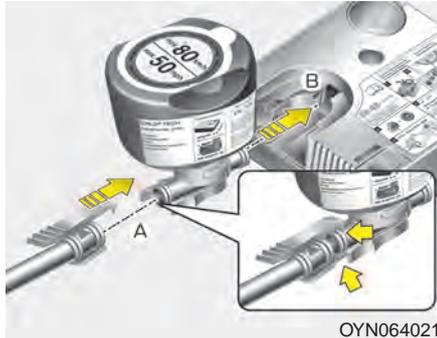
4. Screw the filling hose (a) onto the connector of the sealant bottle (1).
