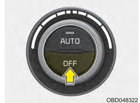
Press the front blower OFF button to turn off the front air climate control system. However, you can still operate the mode and air intake buttons as long as the ignition switch is in the ON position.
