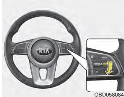
3. Move the lever down (to SET-), and release it at the desired speed. The SET speed on the LCD screen will appear. Release the accelerator at the same time. The desired speed will automatically be maintained.
