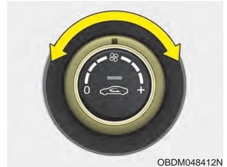
The ignition switch must be in the ON position for fan operation.
