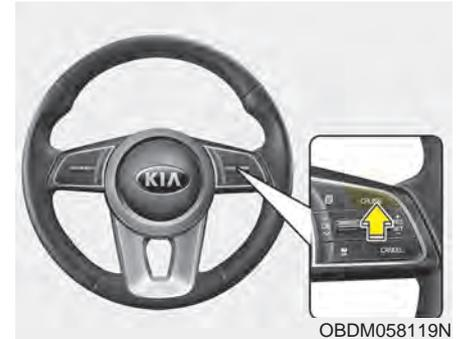
1. Press the CRUISE button to turn the system on. The CRUISE indicator in the instrument cluster will illuminate.
