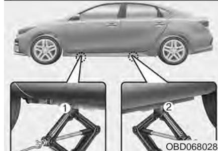
7. Place the jack at the front (1) or rear (2) jacking position closest to the tire you are changing. Place the jack at the designated locations under the frame. The jacking positions are plates welded to the frame with two tabs and a raised dot to line up with the jack.
