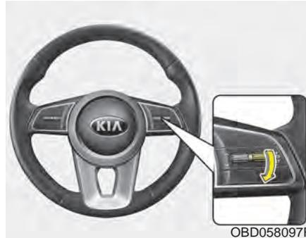
3. Move the lever down (to SET-), and release it at the desired speed. The set speed and vehicle to vehicle distance on the LCD screen will illuminate.
