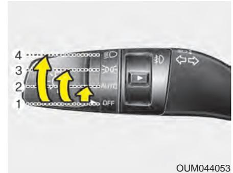
The light switch has a Headlight and a Parking light position.
