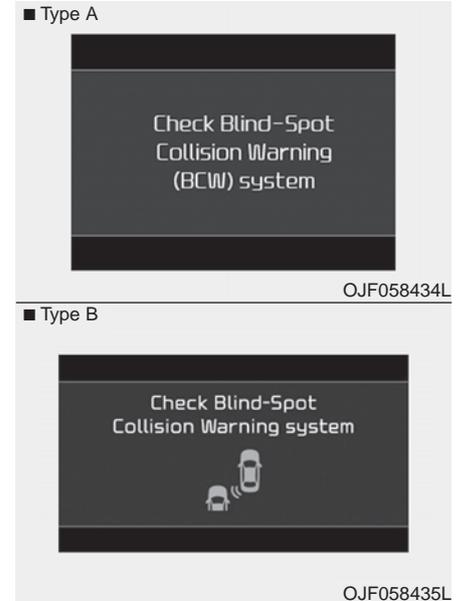
If the system does not work properly, a warning message will appear and the light on the switch will turn off. The system will turn off automatically.
