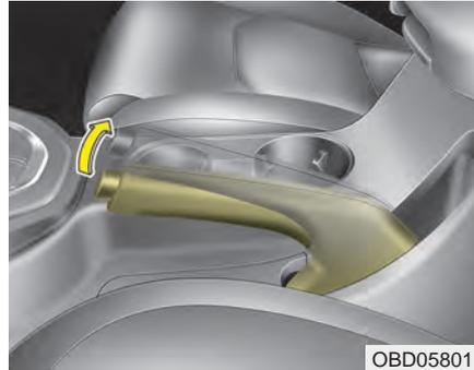
To engage the parking brake, first apply the foot brake and then pull up the parking brake lever as far as possible.
