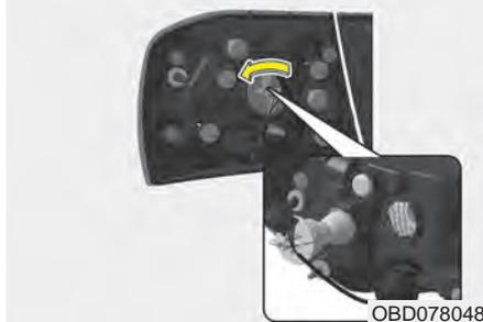
4. Remove the rear combination lamp assembly from the body of the vehicle.
