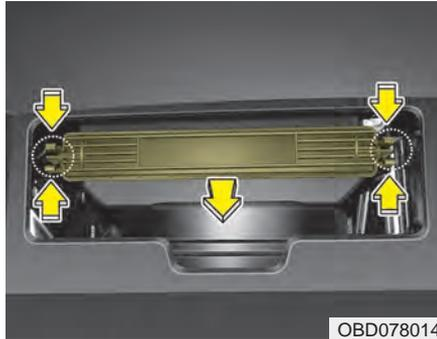
3. Remove the climate control air filter cover while pressing the lock on both sides of the cover.
