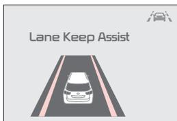
When the LKA-L sensor detects the lanes traveling in, the indicators are illuminated
