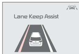
When the LKA-L sensor detects the vehicle moving outside of the lane the vehicle's traveling in, a yellow indicator will illuminate, either on the left or right lane
