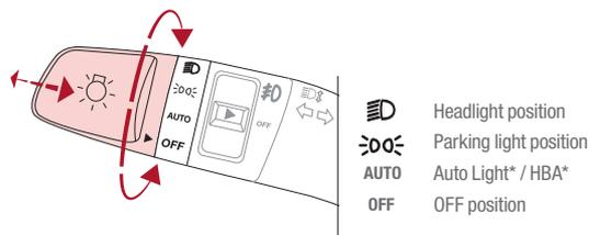
**AUTO Light function\*** — When the light switch is in the AUTO Light position, the tail lights and headlights will turn ON/OFF automatically depending on the amount of light outside the vehicle.
