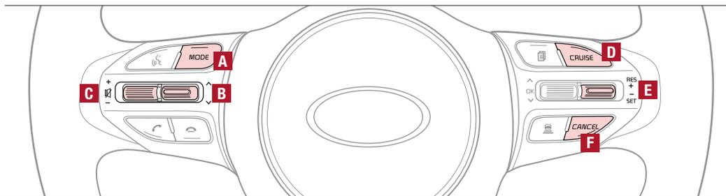
**A Audio MODE button:** Press to cycle through FM/AM/SiriusXM®\*†20/ Media Modes; Audio System ON/OFF: Press to turn power on; Press and hold to turn power off
