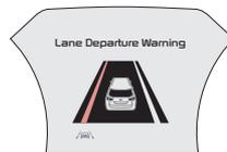
When the LDW sensor detects the vehicle veering outside of the lane traveling in, the lane the vehicle is crossing will blink (shown in both images at left)
