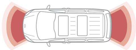
To activate, press button **D** (LED illuminated). The system is also activated when the ignition is ON and the gear shift is moved into R (Reverse). To deactivate the system, press the Parking Distance Warning—Forward\* and Reverse\* button **D** (LED not illuminated).
