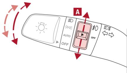
**One-Touch Lane Change Signal** is activated by moving the Turn Signal Lever slightly for less than 1 second and then releasing. The lane change signal will blink 3 times.
