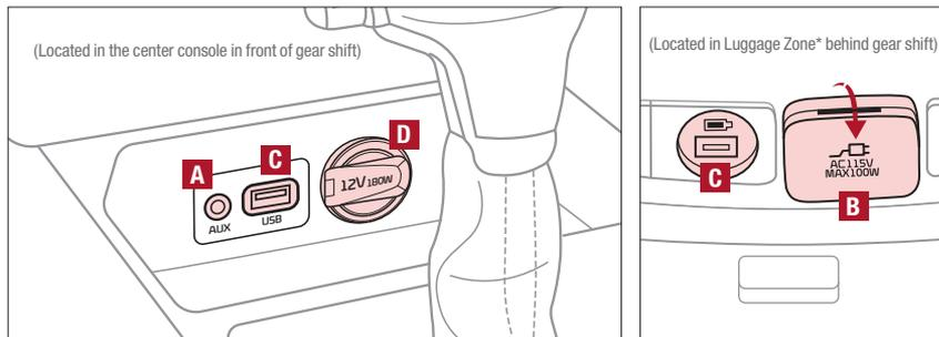
**AUX/Multimedia USB Port A** – Use the AUX port to connect audio devices and the Multimedia USB port to connect USB audio devices and smartphones.
