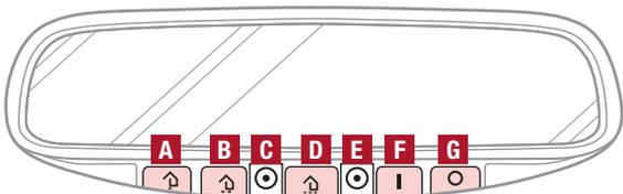
The HomeLink® with Auto-Dimming Rearview Mirror\* is designed to reduce glare from a vehicle's headlights located in the rear and also to connect up to three electronic transmitters into one location.
