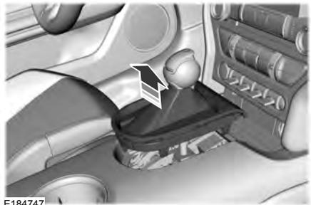
1. Using a flat head screwdriver or similar tool, remove the chrome bezel and gearshift bracket at the base of the gearshift lever.
