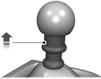
If reverse (R) is not fully engaged, press the clutch pedal down and return the gearshift to the neutral position. Release the clutch pedal for a moment, then raise the collar and shift to reverse (R) again.
