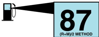
Your vehicle is designed to operate on regular unleaded gasoline with a minimum pump (R+M)/2 octane rating of 87.
