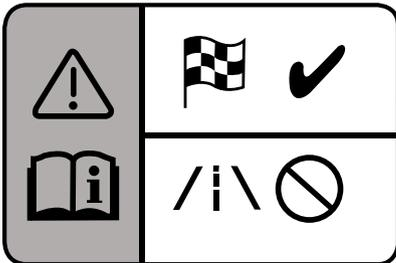
**The rear Gurney flap must be removed for on-road driving.**
