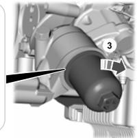
1. Install new O-ring seals on the oil filter housing and lubricate with clean engine oil.
