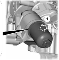
1. Loosen the oil filter housing and allow the oil to drain.
