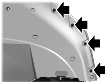
3. Remove the four M6 screws from the outboard corner of the splitter.
