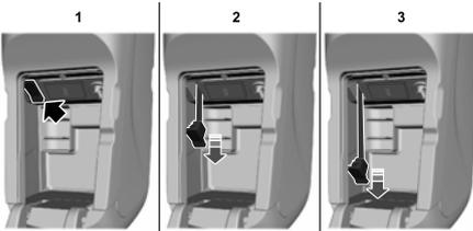
1. Locate the manual park release cable access cover at the bottom of the center storage in the center console.
