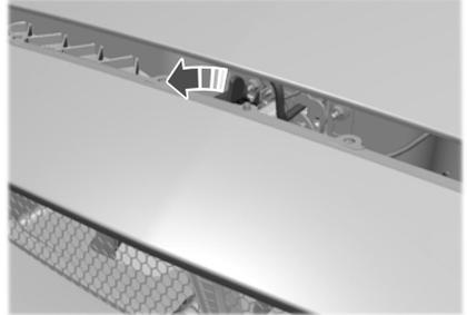
4. Release the hood latch by pushing the secondary release lever to your left-hand side and open the hood.
