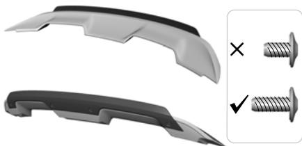
**Note:** The Gurney flap comes with longer size bolts to install it onto the rear spoiler. **Do not use the longer size bolts without the Gurney flap attached or damage to the spoiler may occur.**
