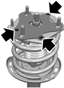
**Note:** The adjustable camber front strut mounts are fitted with three set screws that must be removed before camber can be adjusted. If you cannot adjust the camber, please see your authorized dealer or call 800-367-3788 for more details to remove the set screws.
