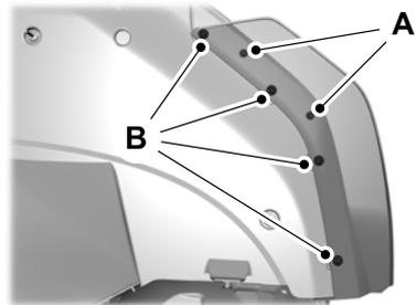
7. Loosely install two M4.2 screws (A) to the bottom of the splitter.
