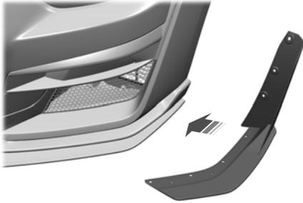
5. Locate the splitter wicker to the vehicle. The face of the splitter wicker with the three attaching holes should be aligned to the wheel liner bracket.
