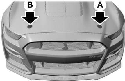
2. Press the driver side hood pin (A) first, then the passenger side hood pin (B).
