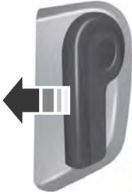
1. Inside the vehicle, pull the hood release handle located under the left-hand side of the instrument panel.
