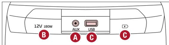
(Ports and power outlets located on lower part of Center Panel; power outlets may be configured differently on your vehicle)
