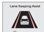
When the front-view camera detects the lane traveling in, both lanes are illuminated
