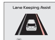
When the front-view camera detects the vehicle veering outside of the lane traveling in, a vehicle crossing lane indicator will illuminate, either on the left or right lane (shown in both images above)
