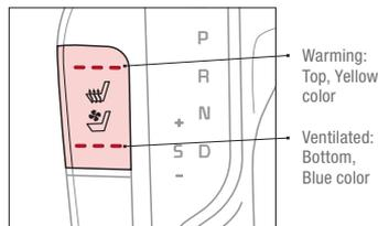
(Buttons located near Gear Shift Lever)
