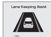
When the front-view camera does not detect the lane traveling in, the lanes are not illuminated
