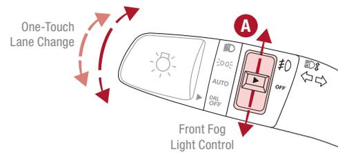
**One-Touch Lane Change Signal** is activated by briefly pressing the Turn Signal lever up/down slightly for less than 1 second and then releasing. The lane change signal will blink 3-7 times.
