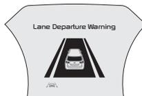
When the LDW sensor does not detect the lane traveling in, the lane is not illuminated
