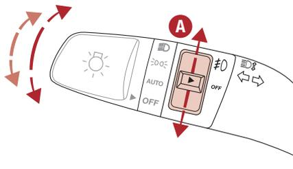
The **One-Touch Lane Change Signal** is activated by briefly pressing the Turn Signal Lever slightly for less than 1 second and then releasing. The lane change signal will blink 3 times.
