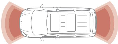
To activate, press button **A** (LED illuminated). The system is also activated when the ignition is ON and the gear shift is moved into R (Reverse). To deactivate the system, press the Parking Distance Warning—Forward\* and Reverse\* button **A** (LED not illuminated).
