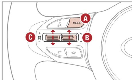
**A Audio MODE button:** Press to cycle through the FM/AM/SiriusXM<sup>®\*\*†20</sup> Media Modes; Audio System ON/OFF: Press to turn the power on
