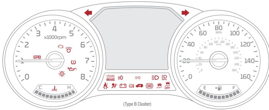
Your vehicle's instrument cluster & indicator light locations may differ from those in the illustrations. For more information on the instrument cluster, the LCD Warning Messages and the function of all indicator and warning lights, please refer to section 2 in the Owner's Manual.
