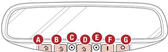
HomeLink® with Auto-Dimming Rearview Mirror\* is designed to reduce glare from a vehicle's headlights located in the rear and also to connect up to three electronic transmitters into one location.
