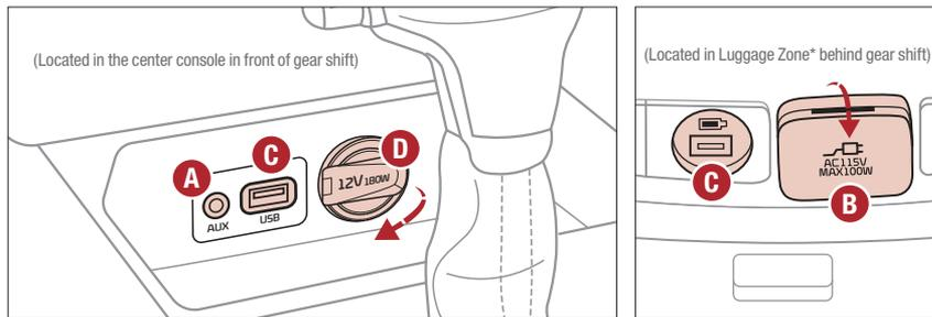
**AUX/Multimedia USB Port A** – Use the AUX port to connect audio devices and the Multimedia USB port to connect USB audio devices and smartphones.
