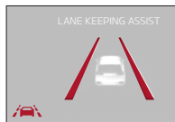
When the front-view camera detects the lane traveling in, both lanes are illuminated
