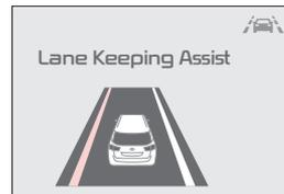
When the front view camera detects the vehicle moving outside of the lane the vehicle's traveling in, a yellow indicator will illuminate, either on the left or right lane
