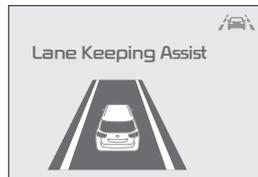
When the front view camera does not detect the lanes traveling in, the indicator will not illuminate
