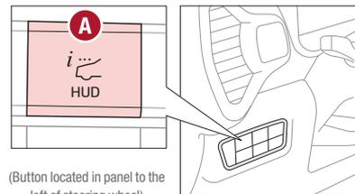
(Button located in panel to the left of steering wheel)
