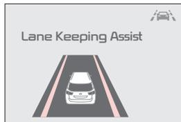
When the front view camera detects the lanes traveling in, the indicators are illuminated
