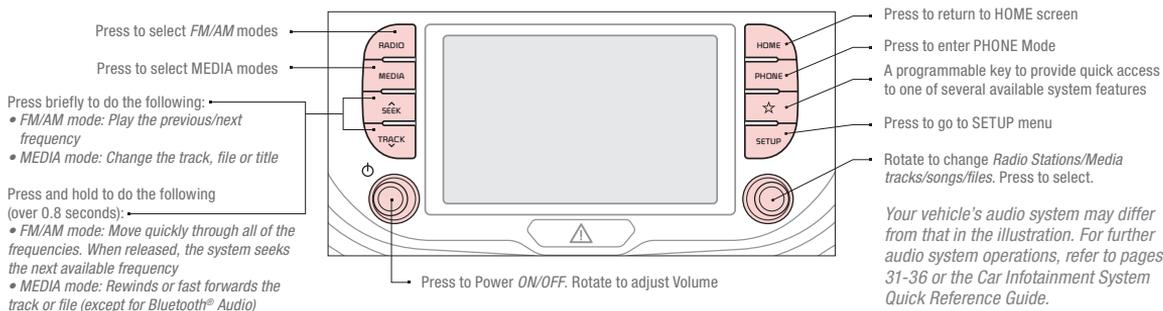
**Audio System Setup Options** – Press the SETUP key, then using the touchscreen, press the menu item to enter (Display, Sound, Clock/Calendar, Phone, System Info). Adjust the available settings for each equipped audio system setup option by pressing the onscreen buttons/arrows. Audio system setup options may include the following:
