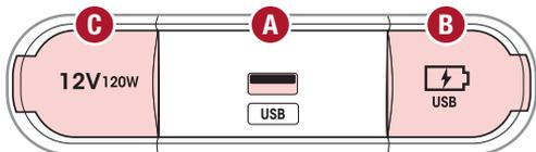
(Ports and power outlets located on lower part of Center Panel; If equipped, an additional Power Outlet is located in the rear cargo area of the vehicle)
