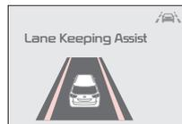
When the front-view camera does not detect the lanes the vehicle is traveling in, the indicator will not illuminate
