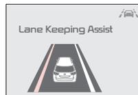
When the front-view camera detects the vehicle moving outside of the lane the vehicle's traveling in, a yellow indicator will illuminate, either on the left or right lane
