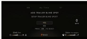
Trailer Blind Spot Information System detects vehicles that may have entered the blind spot zone. The detection area is on both sides of your vehicle and trailer, extending rearward from the exterior mirrors to the end of your trailer.
