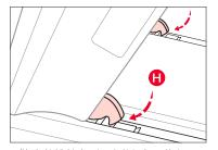
(Hooks highlighted are inserted into channel between bar and white adjustment device)
