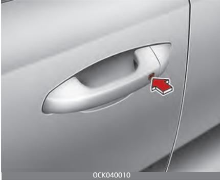
Pressing the button of the front outside door handles with all doors closed and any door unlocked, locks all the doors. The hazard warning lights will blink and the chime will sound once to indicate that all doors are locked. The button will only operate when the smart key is within 28~40 in. (0.7~1 m) from the outside door handle. If you want to make sure that a door has locked or not, you should check the door lock button inside the vehicle or pull the outside door handle.
