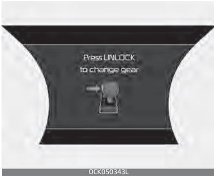
The warning message appears on the LCD display, when the [UNLOCK] button is not pressed while shifting the gear.
