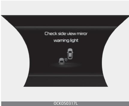
When the side view mirror (outside mirror) warning light is not working properly, the 'Check side view mirror warning light' warning message will appear on the cluster. In this case, have your vehicle inspected by an authorized Kia dealer.
