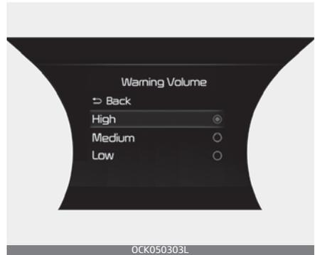
With the ENGINE START/STOP button in the ON position, select 'Driver Assistance → Warning Volume' from the "User Settings (LCD display) or Setup → Vehicle (Infotainment System screen)" to change the Warning Volume to 'High', 'Medium', 'Low' for Blind-Spot Safety system.
