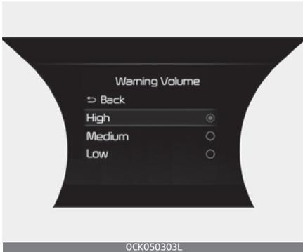
With the ENGINE START/STOP button in the ON position, select 'Driver Assistance → Warning Volume' from the "User Settings (LCD display) or Setup → Vehicle (Infotainment System screen)" to change the warning volume to 'High', 'Medium', 'Low' for Highway Driving Assist.
