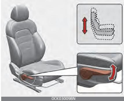
To change the height of the seat cushion, push the lever that is located on the outside of the seat cushion upwards or downwards.
