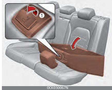
5. To use the rear seat, lift and push the seatback backward. Push the seat back firmly until it clicks into place. Make sure the seatback is locked in place.
