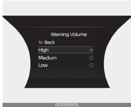
With the ENGINESTART/STOP button in the ON position, select ‘Driver Assistance → Warning Volume’ from the “User Settings (LCD display) or Setup → Vehicle (Infotainment System screen)” menu to change the Warning Volume to ‘High’, ‘Medium’, ‘Low’ for Smart Cruise Control.
