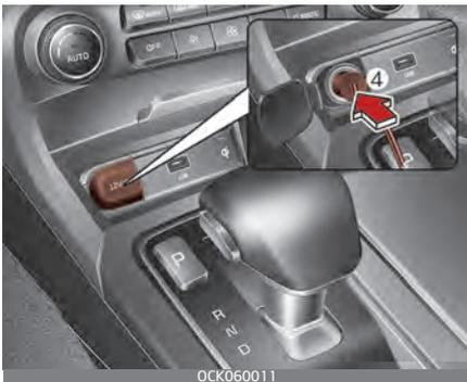
10. With the ENGINE START/STOP button position on: switch on the compressor and let it run for approximately 5~7 minutes to fill
