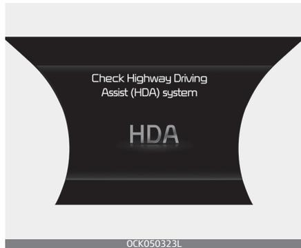
When Highway Driving Assist is not working properly, the 'Check Highway Driving Assist (HDA) system' warning message will appear, and the (⚠️) warning light will illuminate on the cluster.
