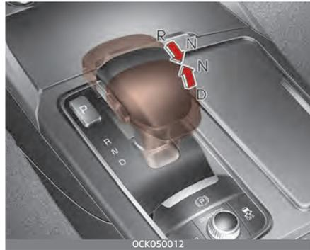
The wheels and transmission are not engaged.
