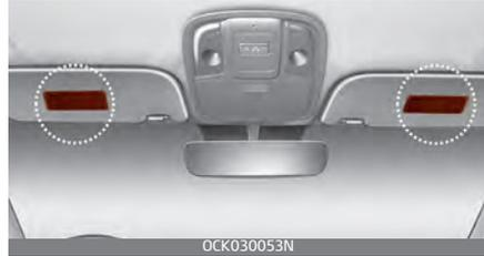
Air bag warning labels, some required by the U.S. National Highway Traffic Safety Administration (NHTSA), are attached to the sunvisor to alert the driver and passengers of potential risks of the air bag system.
