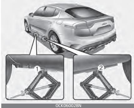
8. Insert the wheel lug nut wrench into the jack and turn it clockwise, raising the vehicle until the tire just clears the ground. This measurement is approximately 1 in (30 mm). Before removing the wheel lug nuts, make sure the vehicle is stable and that there is no chance for movement or slippage.
