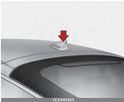
The shark fin antenna will receive both AM and FM signals and the transmit data.
