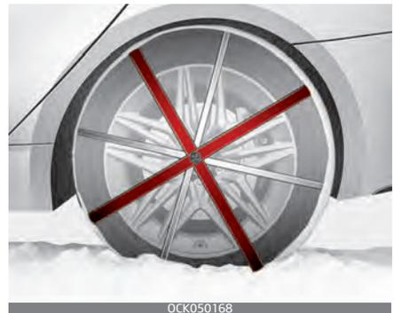
Since the sidewalls on some radial tires are thinner than other types of tires, they may be damaged by mounting certain types of tire chains on them. Therefore, the use of snow tires is recommended instead of tire chains. Do not mount tire chains on vehicles equipped with aluminum wheels; if unavoidable,
