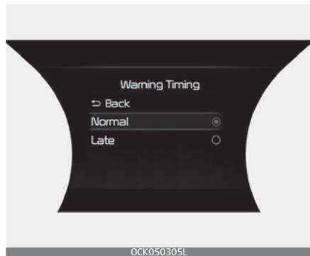
With the ENGINE START/STOP button in the ON position, select 'Driver Assistance → Warning Timing' from the "User Settings (LCD display) or Setup → Vehicle (Infotainment System screen)" menu to change the initial warning activation time for Rear Cross-Traffic Safety system.
