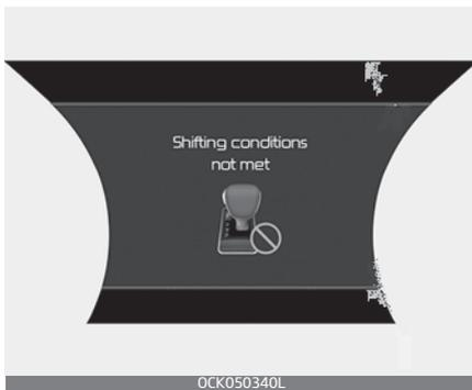
The warning message appears on the LCD display, when engine RPM is too high, or when driving speed is too fast to shift the gear.
