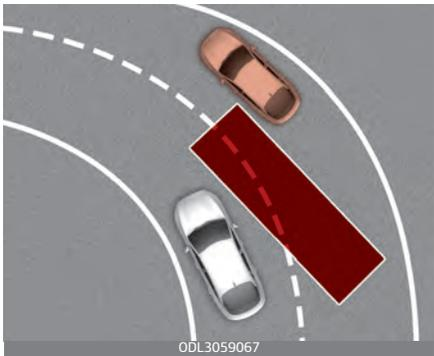
Blind-Spot Safety system may not operate properly when driving on a curved road. The function may not detect the vehicle in the next lane. Always pay attention to road and driving conditions while driving.
