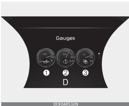
This mode displays Oil temperature (1), Torque gauge (2), Turbo boost gauge (3).
