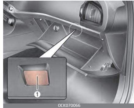
If the glove box lamp (LED) (1) does not operate, have the vehicle checked by an authorized Kia dealer.
