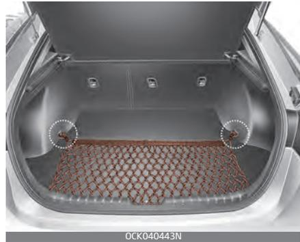
To keep items from shifting in the cargo area, you can use the holders located in the cargo area to attach the luggage net. (if equipped)
