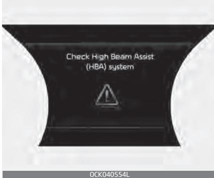
When High Beam Assist is not working properly, the 'Check High Beam Assist (HBA) system' warning message will appear on the cluster (turns off after a certain time) and (⚠) warning light will illuminate.
