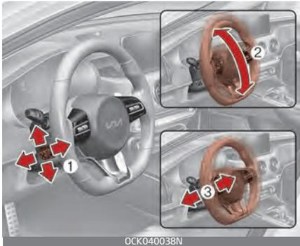
After adjusting, push the steering wheel both up and down to be certain it is locked in position. Always adjust the position of the steering wheel before driving.
