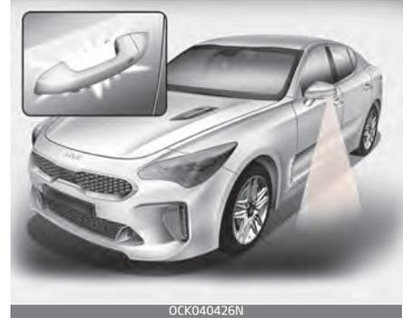
When all the doors (and liftgate) are locked and closed, the pocket lamp and puddle lamp, room lamp will come on for about 15 seconds if any of the below is performed.
