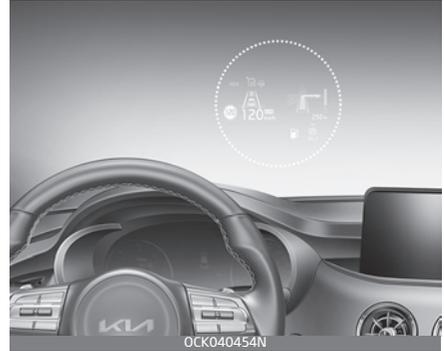
The Head Up Display is a transparent display which projects some information of the instrument cluster and navigation on the windshield glass.
