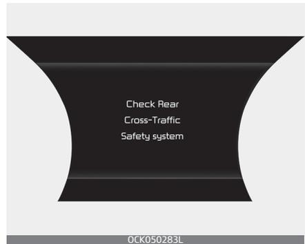
When Rear Cross-Traffic Safety system is not working properly, the 'Check Rear Cross-Traffic Safety system' warning message will appear on the cluster, and the function will turn off automatically or the function will be limited. In this case, have your vehicle inspected by an authorized Kia dealer.
