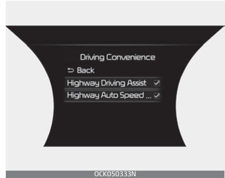
With the ENGINE START/STOP button in the ON position, select 'Driver Assistance → Driving Convenience' from the setting menu to set whether or not to use each function.
