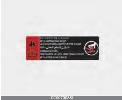
Do not touch metal parts (including strut bars) while the engine is operating or hot. Doing so could result in serious personal injury. Turn the engine off and wait until the metal parts cool down to perform maintenance work on the vehicle.
