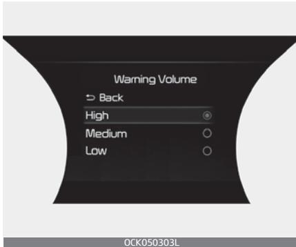
With the ENGINE START/STOP button in the ON position, select 'Driver Assistance → Warning Volume' from the 'User Setting (LCD display) or Setup → Vehicle (Infotainment System screen)' to change the Warning Volume to 'High', 'Medium' or 'Low' for Hands-off warning.
