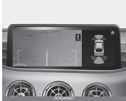
When you touch the Soft button (1), the top view is displayed on the screen and shows the distance from the vehicle in the back of your vehicle while parking.
