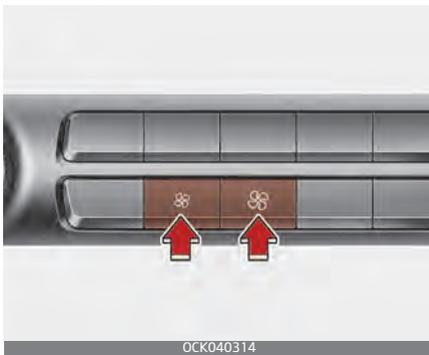
The fan speed can be set to the desired speed by pushing the fan speed control button.
