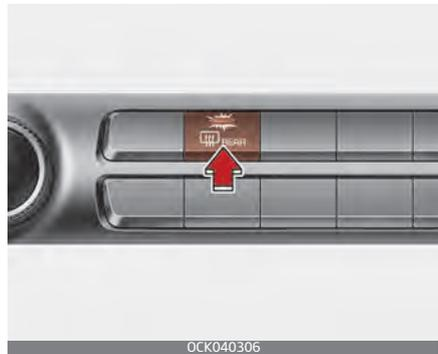
The defroster heats the window to remove frost, fog and thin ice from the rear window, while the engine is running.
