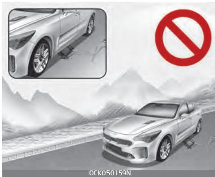
Never start or run the engine while an AWD vehicle is raised on a jack. The vehicle can slip or roll off of a jack causing serious injury or death to you or those nearby.
