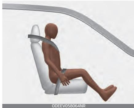
When an adult is seated in the front passenger seat, if the PASSENGER AIR BAG "OFF" indicator is on, turn the Engine Start/Stop button to the OFF position and ask the passenger to sit properly (sitting upright with the seat back in an upright position, centered on the seat cushion with their seat belt on, legs comfortably extended and their feet on the floor). Restart the engine and have the person remain in that position.
