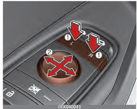
The electric remote control mirror switch allows you to adjust the position of the left and right outside rearview mirrors. To adjust the position of either mirror, press the R or L button (1) to select the right side mirror or the left side mirror, then press a corresponding point (▲) (2) on the mirror adjustment control to position the selected mirror up, down, left or right.
