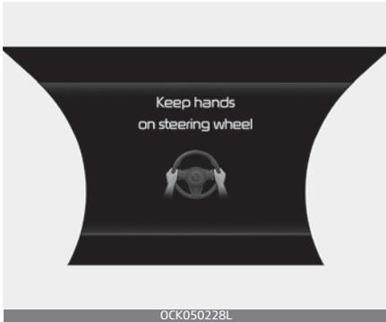
The hands-off warning appears when the function detects that the driver's hands are not on the steering wheel while HDA is in work.
