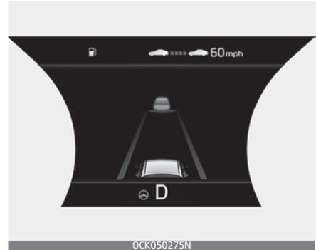
If the vehicle ahead or both lane markings are detected and your vehicle speed is below 120 mph (200 km/h), the green (🚗) indicator light will illuminate on the cluster, and the function will help the vehicle stay in lane by controlling the steering wheel.
