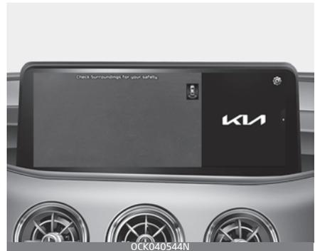
Rear view while driving is a driving assist function that shows the image behind the vehicle on the
