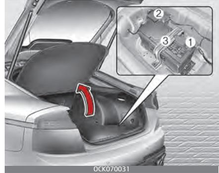
The battery is in the trunk under the compartment cover.
