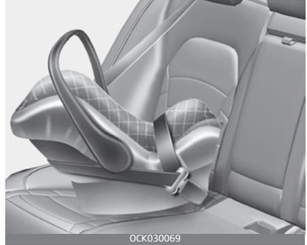
A rear-facing child seat provides restraint with the seating surface against the back of the child. The harness system holds the child in place, and in an accident, acts to keep the child positioned in the seat and reduces the stress to the neck and spinal cord.
