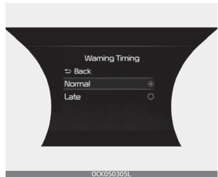
The driver can select the initial warning activation time in the User Settings in the LCD display by selecting "User Settings (LCD display) or Setup → Vehicle (Infotainment System screen) → Driver Assistance → Warning Timing". When the vehicle is first delivered, warning timing is set to 'Normal'. If
