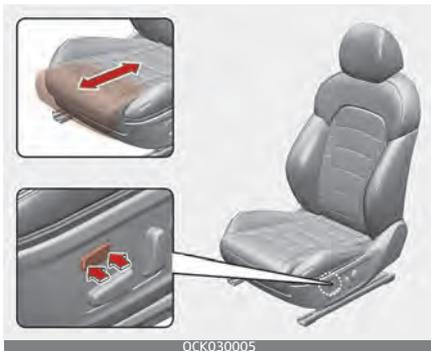
1. Push the front part of control switch to move the seat cushion to the desired length.
