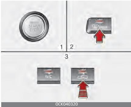
1. Turn the ENGINE START/STOP button to the ON position.
