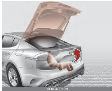
If, during power opening or closing, the liftgate is blocked by an object or part of someone’s body, the power liftgate will detect the resistance and it will stop movement or move to the full open position to allow the object to be cleared.
