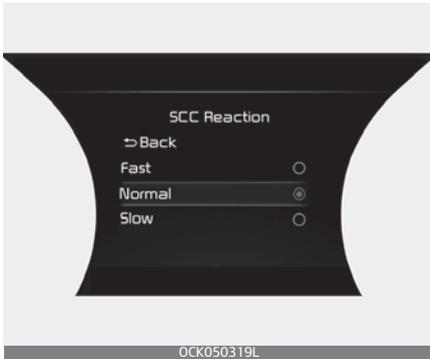
The sensitivity of vehicle speed when following the front vehicle to maintain the set distance can be adjusted. Go to the “User Settings (LCD display) or Setup → Vehicle (Infotainment System screen)” menu to change the Warning Volume to ‘High’, ‘Medium’, ‘Low’ for Smart Cruise Control. You may select one of the three stages you prefer.
