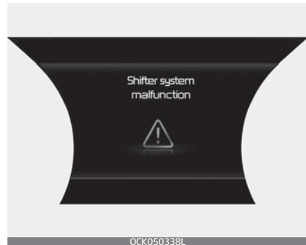
The warning message appears on the LCD display, when the transmission or the shift lever does not properly operate in the P (Park) position. In this case, have the vehicle inspected by an authorized Kia dealer immediately.
