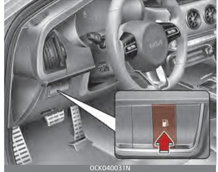
The fuel filler door must be opened from inside the vehicle by pressing the fuel filler door opener button.
