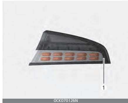
If the rear side marker (LED) (1) does not operate, have the vehicle checked by an authorized Kia dealer.
