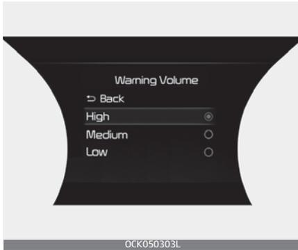
With the ENGINE START/STOP button in the ON position, select 'Driver Assistance → Warning Volume' from the "User Settings (LCD display) or Setup → Vehicle (Infotainment System screen)" menu to change the Warning Volume to 'High', 'Medium', 'Low' for Rear Cross-Traffic Safety system.
