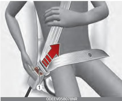
The seat belt is released by pressing the release button (1) in the locking buckle. When it is released, the belt should automatically draw back into the retractor.
