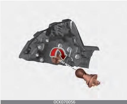
8. Remove the bulb from the socket by pressing it in and rotating it counterclockwise until the tabs on the bulb align with the slots in the socket. Pull the bulb out of the socket.
