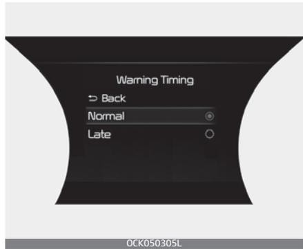
With the ENGINE START/STOP button in the ON position, select 'Driver Assistance → Warning Timing' from the "User Settings (LCD display) or Setup → Vehicle (Infotainment System screen)" menu to change the initial warning activation time for Forward Collision-Avoidance Assist.
