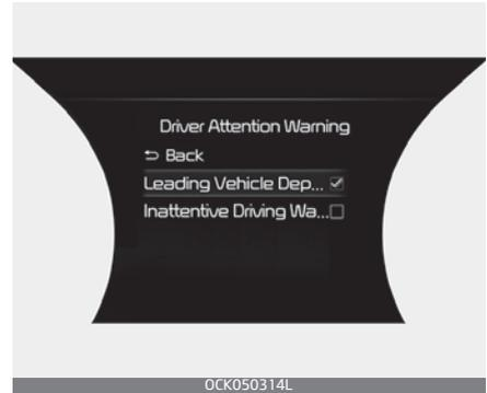
If 'Leading Vehicle Departure Alert' is selected, the function will inform the driver when the front vehicle departs from a stop.
