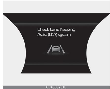
When Lane Keeping Assist is not working properly, the 'Check Lane Keeping Assist (LKA) system', warning message will appear and the yellow (
