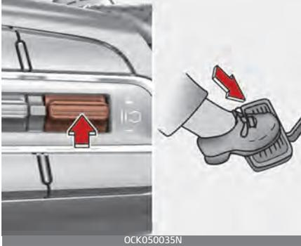
Press the || ↻ switch or depress the brake pedal to temporarily cancel Smart Cruise Control.
