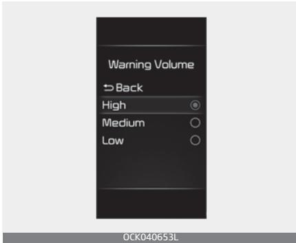
With the ENGINE START/STOP button in the ON position, and select 'User Settings (LCD display) or Setup → Vehicle (Infotainment System screen) → Driver Assistance → Warning Volume' to change the warning volume to 'High', 'Medium' or 'Low' for Blind-Spot Safety system.
