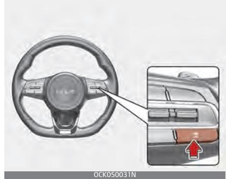
Each time the Vehicle Distance button is pressed, the Vehicle Distance changes as follows:
