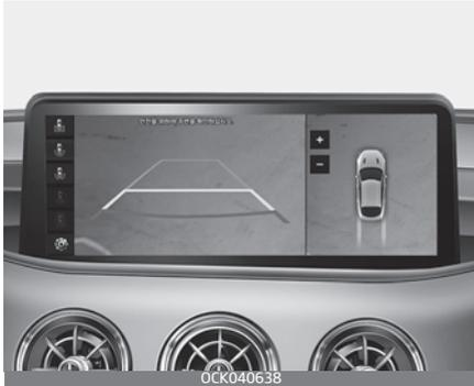
Surround View Monitor can assist in parking by allowing the driver to see around the vehicle.
