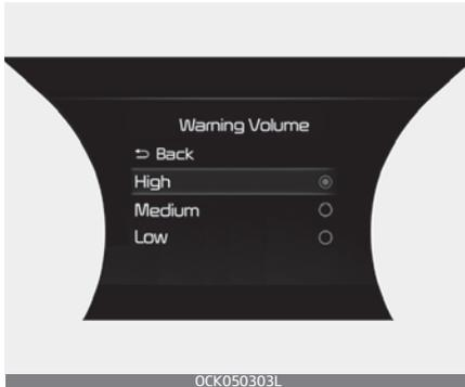
With the ENGINE START/STOP button in the ON position, select 'Driver Assistance → Warning Volume' from the "User Settings (LCD display) or Setup → Vehicle (Infotainment System screen)" to change the Warning Volume to 'High', 'Medium', 'Low' for Lane Keeping Assist.
