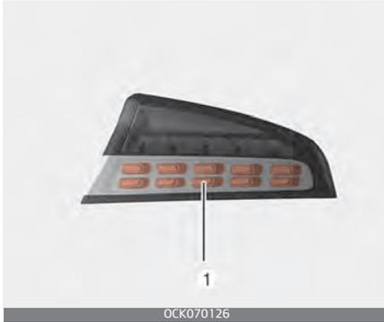
If the rear turn signal lamp (LED) (1), does not operate, have the vehicle checked by an authorized Kia dealer.
