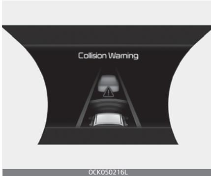
While Smart Cruise Control is operating, when the collision risk with the vehicle ahead is high, the 'Collision Warning' warning message will appear on the cluster, and an audible warning will sound to warn the driver. Always have your eyes on the road while driving, and if necessary, depress the brake pedal to reduce your driving speed in order to maintain a safe distance.
