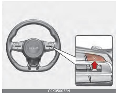
Press the Driving Assist
