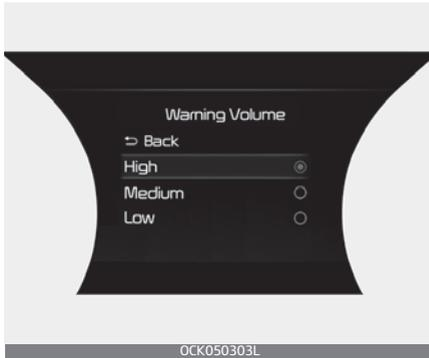
With the ENGINE START/STOP button in the ON position, select 'Driver Assistance → Warning Volume' from the "User Settings (LCD display) or Setup → Vehicle (Infotainment System screen)" menu to change the Warning Volume to 'High', 'Medium', 'Low' for Forward Collision-Avoidance Assist.
