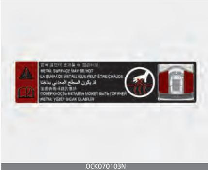
Do not touch metal surfaces in the trunk under the compartment cover while the engine is operating or hot. Doing so could result in serious personal injury.
