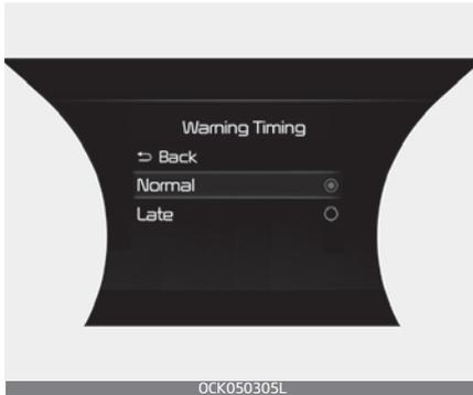
With the ENGINE START/STOP button in the ON position, select 'Driver Assistance → Warning Timing' from the "User Settings (LCD display) or Setup → Vehicle (Infotainment System screen)" to change the initial warning activation time for Blind-Spot Safety system.
