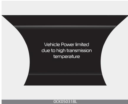
This message is displayed when the transmission oil temperature is high. Drive at steady speed or stop the vehicle at a safe place with the engine on. When the oil temperature returns to normal, the message will disappear.
