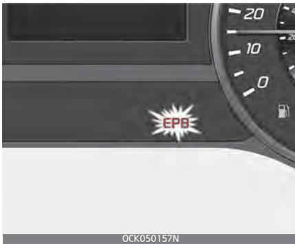
This warning light illuminates if the ENGINE START/STOP button is changed to the ON position and goes off in approximately 3 seconds if the system is operating normally.
