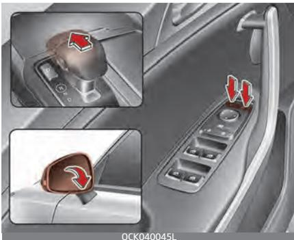
While the vehicle is moving in reverse, the outside rearview mirror(s) will tilt downward to aid reverse parking. According to the position of the outside rearview mirror switch, the outside rearview mirror(s) will operate as follows:
