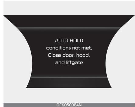
When you press the [AUTO HOLD] switch, if the driver's door and engine hood are not closed or the driver's seat belt is unfastened, a warning will sound and a message will appear on the LCD display. At this moment, press the [AUTO HOLD] button after closing the driver's door and engine hood and fastening the seat belt.
