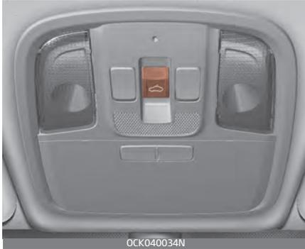
You can operate the sunroof with the sunroof switch in the ignition ON position.
