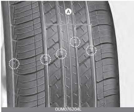
If the tire is worn evenly, a tread wear Indicator (A) will appear as a solid band across the tread. This shows there is less than 1/16 inch (1.6 mm) of tread left on the tire. Replace the tire when this happens.
