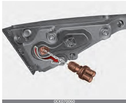
8. Insert a new bulb by inserting it into the socket and rotating it until it locks into place.
