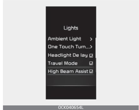
By selecting as 'User Settings (LCD display) or Setup → Vehicle (Infotainment System screen) → Lights → High Beam Assist' on the cluster LCD display or the Infotainment System screen at engine ON, you may select or release the function. The settings will remain even if engine OFF and ON.
