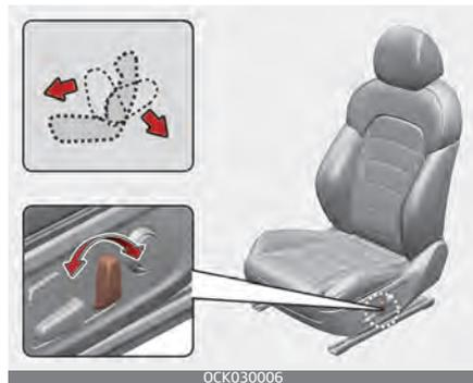
Push the control switch forward or backward to move the seatback to the desired angle. Release the switch once the seat reaches the desired position.
