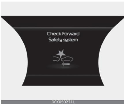
When Forward Collision-Avoidance Assist is not working properly, the 'Check Forward Safety system'
