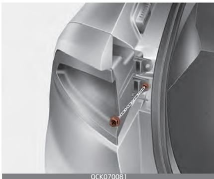
4. Remove the garnish (1) on the top of the rear combination lamp and loosen the 1 screw (2) on the top.
