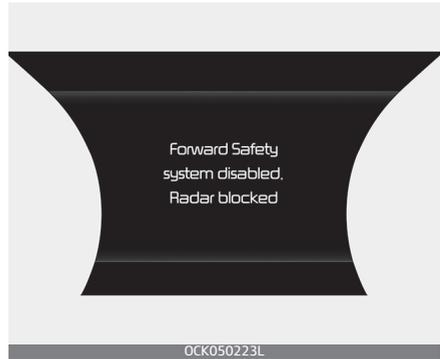
When the front windshield where the front view camera is located, front radar cover or sensor is covered with foreign material such as snow or rain, it can reduce the detecting performance and temporarily limit or disable Forward Collision-Avoidance Assist. If this occurs the 'Forward Safety system dis-
