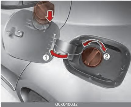
4. To remove the cap, turn the fuel filler cap (2) counterclockwise.
