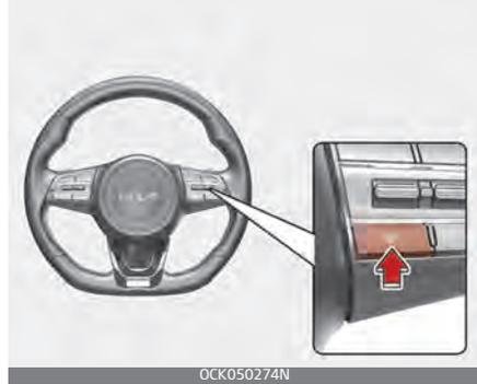
To activate/deactivate LKA, with the ENGINE START/STOP button in the ON position, press and hold the Lane Driving Assist button (
