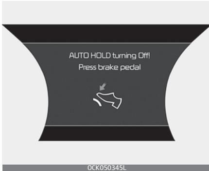
When the conversion from Auto Hold to EPB is not working properly a warning will sound and a message will appear.
